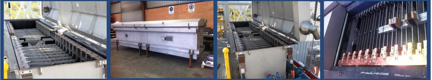
*Como Engineers Pty Ltd are suppliers of heavy duty 304 Stainless steel, rubber lined electrowinning cells. These are applicable to use for the recovery of precious metals.*
